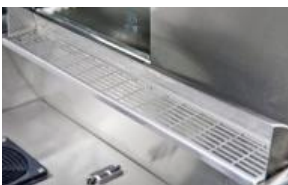
Blown air units circulate above and below the pans
