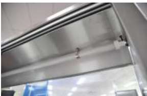
Top mounted fluorescent lighting
