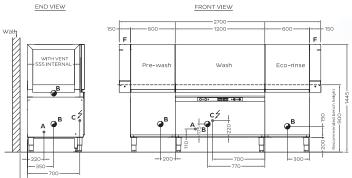
Recommended minimum of 100mm in which case all services can be located centred 50mm off wall, and bench depth = 750mm. Gap to wall may be reduced to 75mm and bench to 700mm but services must then come through floor in adjacent location as shown.
