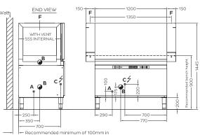
which case all services can be located centred 50mm off wall, and bench depth = 750mm. Gap to wall may be reduced to 75mm and bench to 700mm but services must then come through floor in adjacent location as shown.
